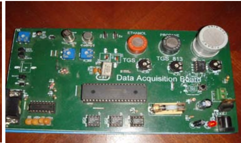
Fig. 1-b. Electronic nose of gas detection without chamber
