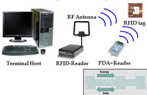
Fig. 2. Usual components of a RFID system
