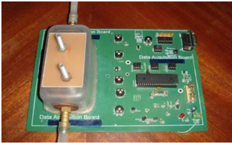
Fig. 1-a. Electronic nose of gas detection with chamber
